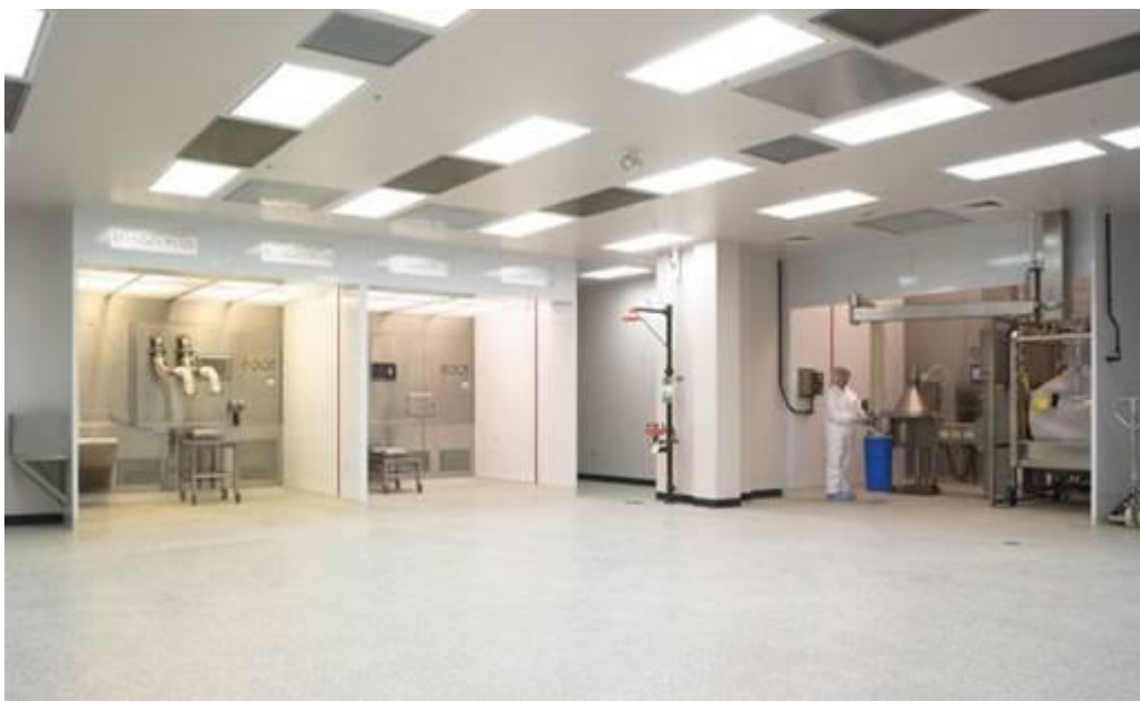
Figure 10-1. Dispensing booths prevent cross-contamination
