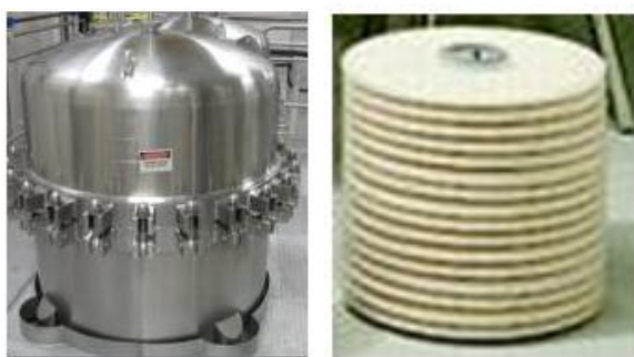
Figure 10-34. A depth filter housing and internal filter stack
